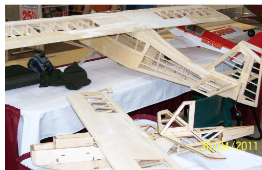
Cliff's Dynaflyte "Decathlon" kit in bare bones condition
