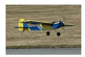
For this months Plane of the Month I am going to pick on roger again with his beautifully built GOLDFINCH. He built it all by hand from a kit, you don't see that much anymore. From Mr aerodesign. It Has a 55 inch wingspan with a 43 inch overall length, Weighing 3 to 4 pounds when finished it takes a 4 channel radio and takes a 40-46 engine We have all seen roger fly it and can see it fly's beautifully. Nice job roger
